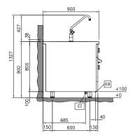
CWII = Cold Water inlet 1 (cleaning) FI Electrical inlet (power) EQ Equipotential screw Hot water inlet
